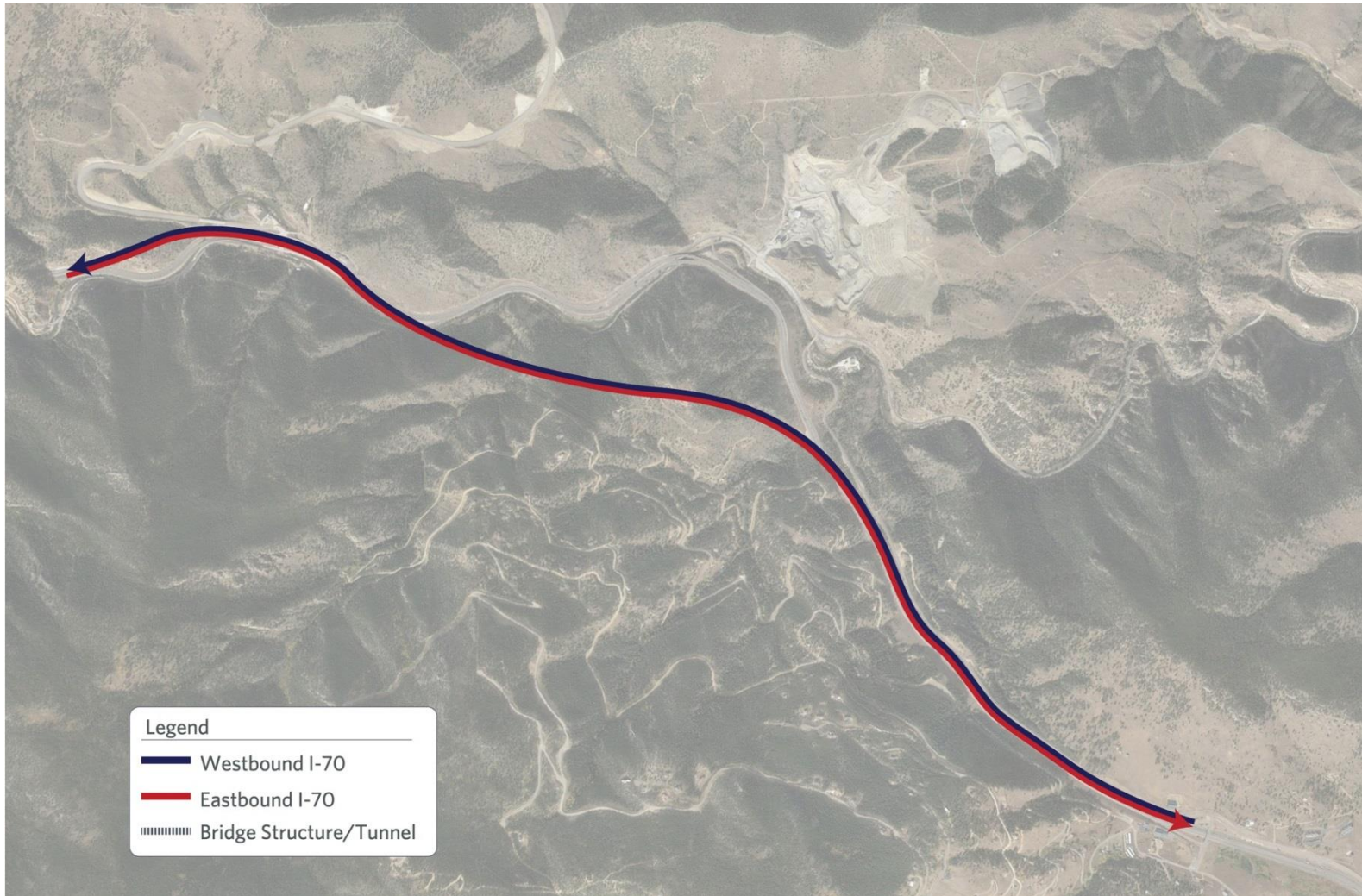
Figure 8. Placing EB and WB Alignments in a Tunnel Located Under the Landslide (NOT RECOMMENDED)
