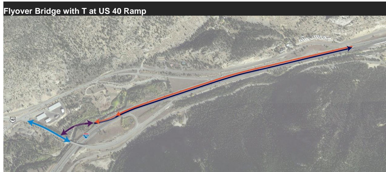
Figure 23. Interchange Concept at Empire Junction—T Junction
